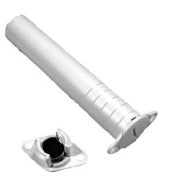
The RF3402 Recessed Wireless Magnetic Contact is a radio frequency (RF) wireless transmitter supplying concealed protection on doors or windows. A Lexan<sup>®</sup> cylinder enclosure designed for durability houses the transmitter and provides tamper protection. You can surface mount or remove the break-away tabs to flush mount the transmitter and magnet assembly.
